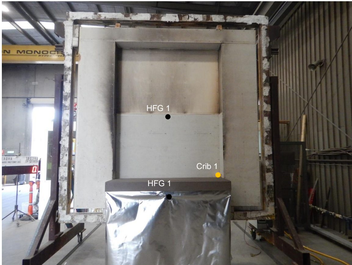
Figure 4 Indicative heat flux gauge locations (exposed side shown)
