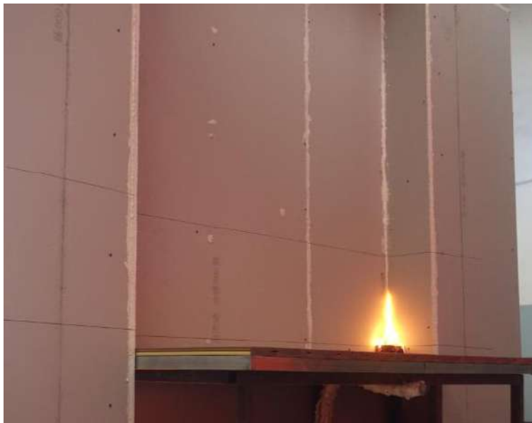
Fig. 2 Exposed Side during the radiant heat test
