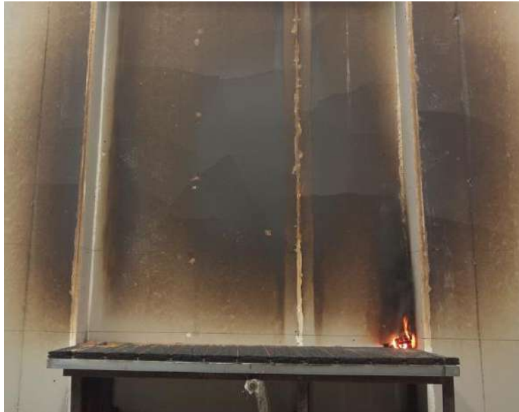
Fig. 3 Exposed Side after the radiant heat test
